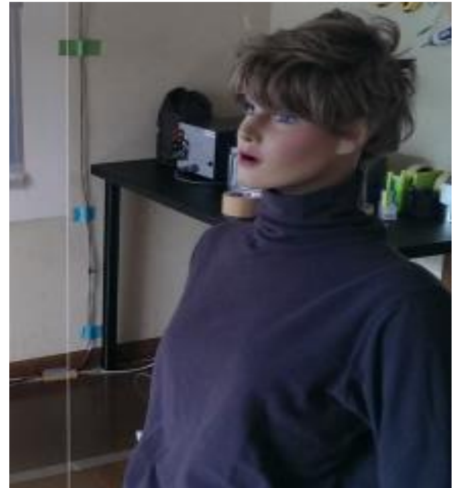
Figure 9 Thermal mannequin clothing sitting position
