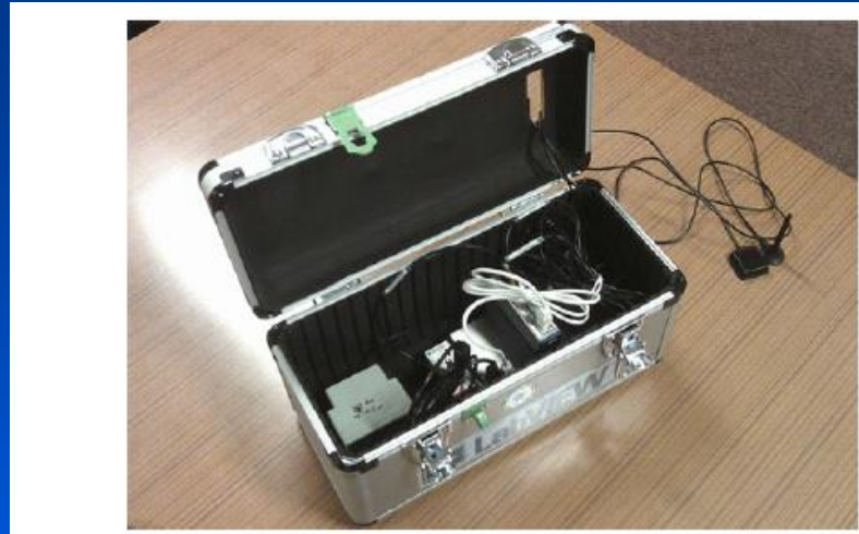
Fig. 7.5 In-vehicle unit of KURAMA-II. A CsI detector and a CompactRIO are compactly placed in a tool box 34.5×17.5×19.5 cm in size
